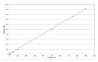
Fig. 9 - Comparison between sample turbidity and turbidity measured using TurbSense with samples with a wide range of turbidities.
