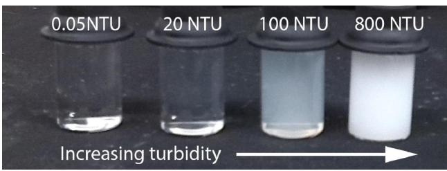
Fig. 1 - Examples of solutions with different turbidities.
