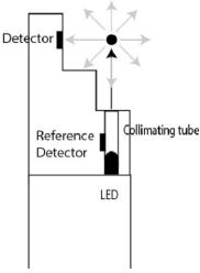
Fig. 2 - Illustration of Pi's TurbSense probe.
